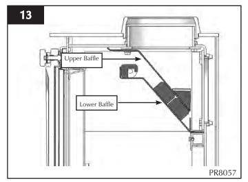
5.3 Remove **the Lower Baffle** (see diagram) by lifting the front edge to unhook it from the support bars
